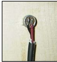
Microphone, glued to the back of the wall
